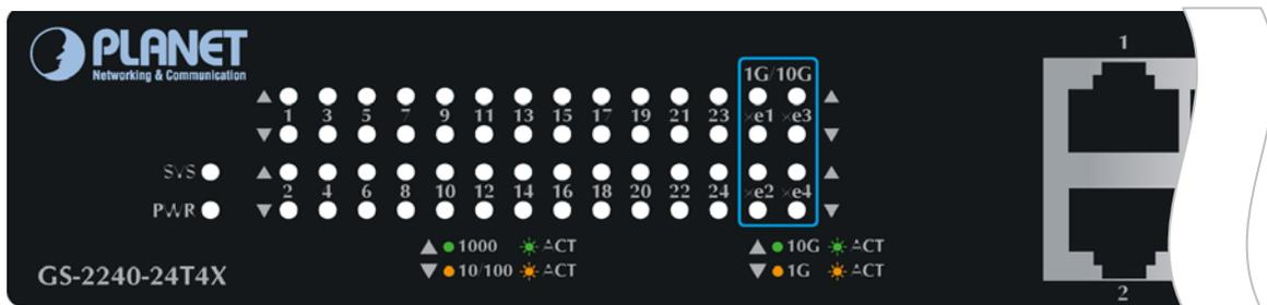
Figure 2-1-3: GS-2240-24T4X LED on Front Panel
