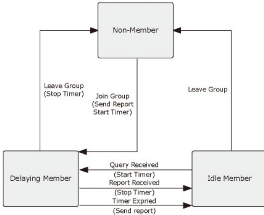
Figure 4-7-1-4 IGMP State Transitions
