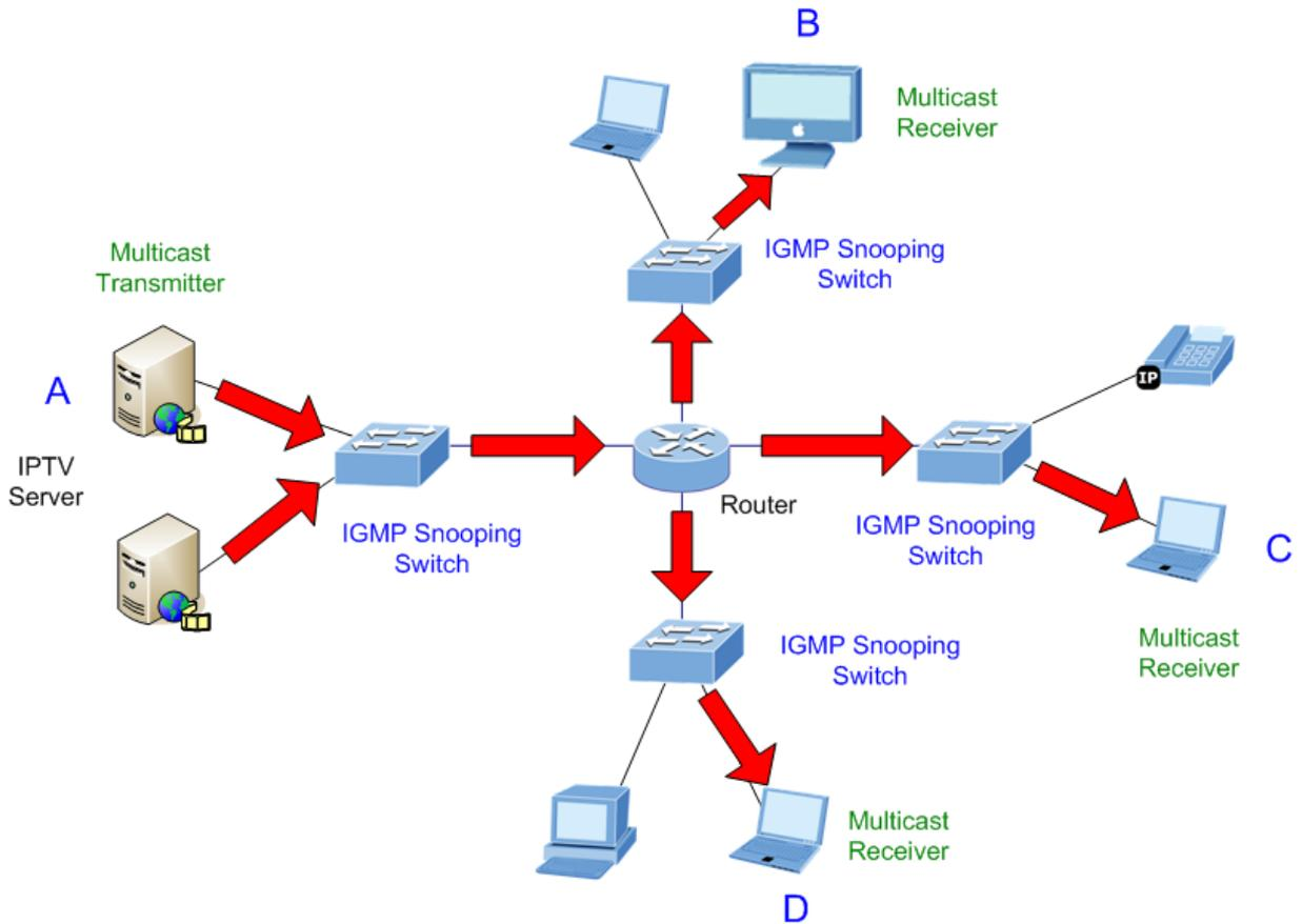
Figure 4-7-1-3 IGMP Snooping Multicast Stream Control
