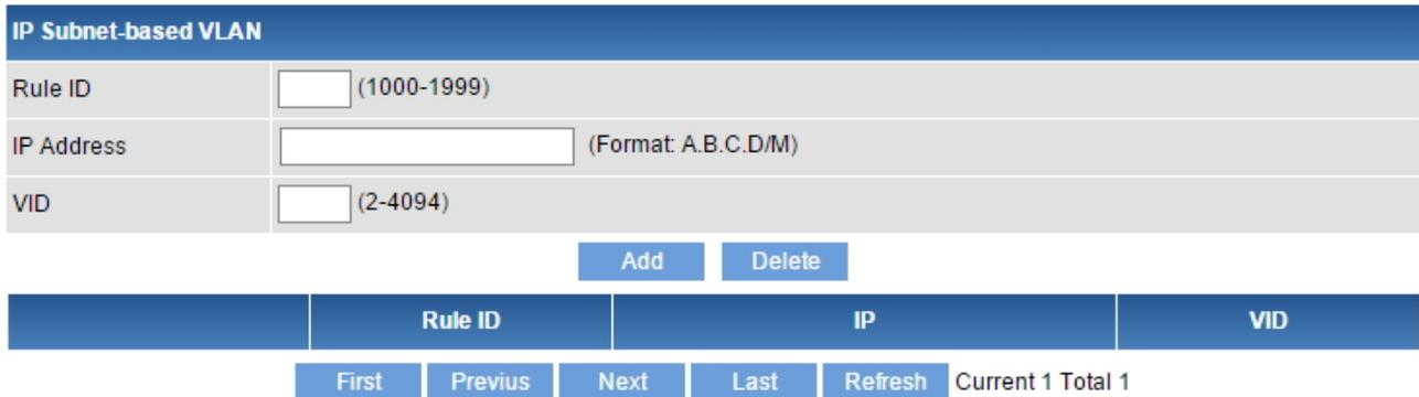
**Figure 4-5-5:** IP Subnet-based VLAN Configuration Page Screenshot
