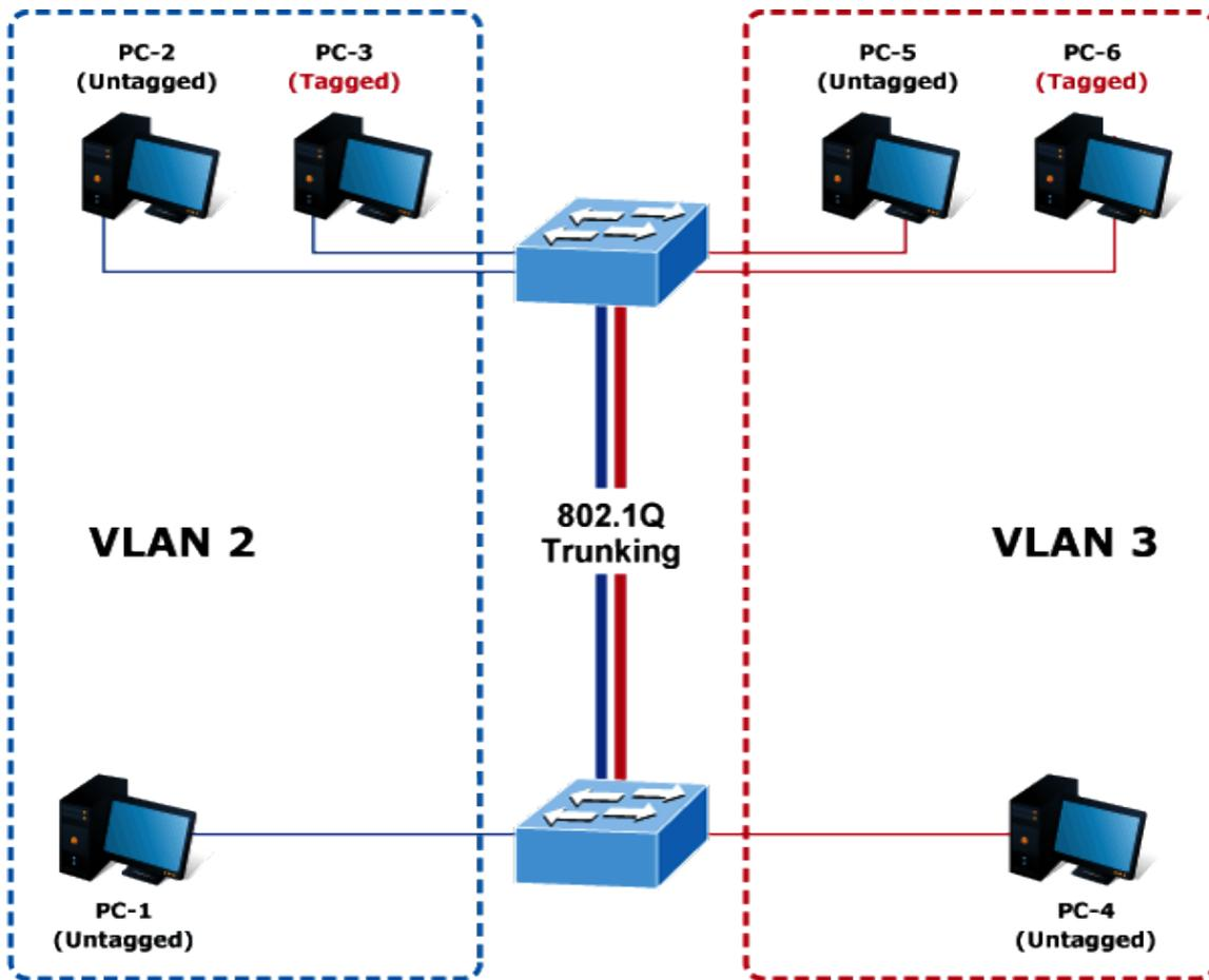
Figure 4-5-21 VLAN Trunking between Two 802.1Q Diagrams
