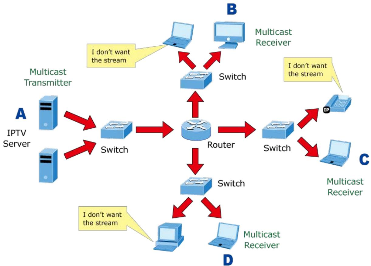
Figure 4-7-1-2 Multicast Flooding
