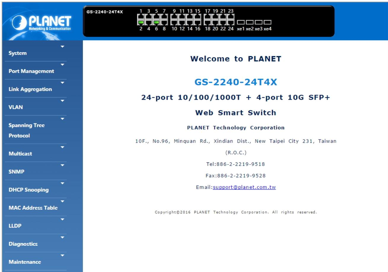
Figure 3-1-4: Web Main Screen of Managed Switch
