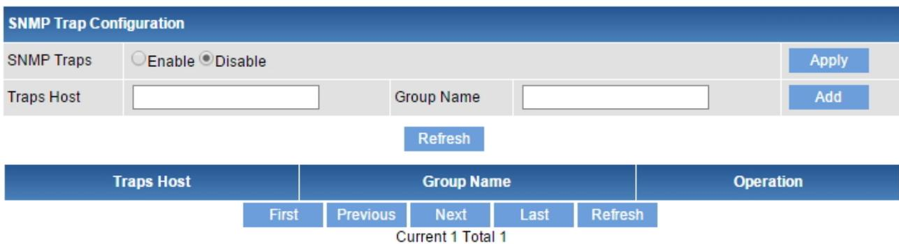
**Figure 4-8-4:** SNMP Trap Configuration Page Screenshot
